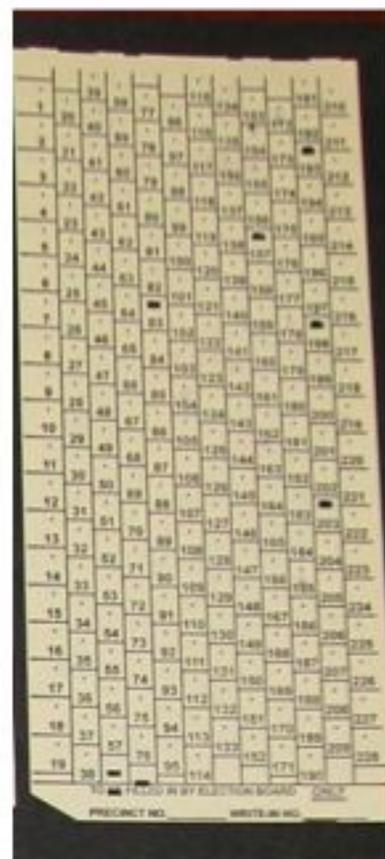
**THIS BALLOT WAS PLACED BACKWARDS. ONLY HALF THE COLUMNS ALIGNED WELL ENOUGH TO BE PUNCHED. THE VOTER INTENT WAS #21, #26, #31, #62 AND #140.**
